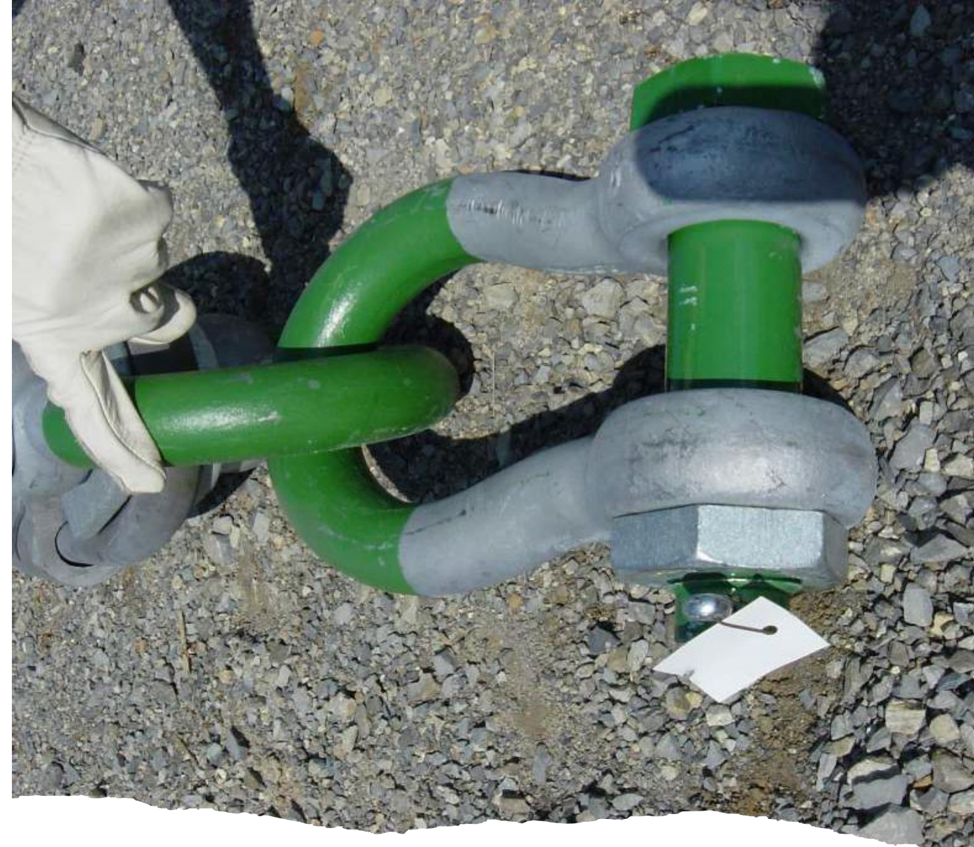
Guyed-V tower: Anchor shackle used for guywire attachment – 135 lb. Example – 765kV Large Scale Components
